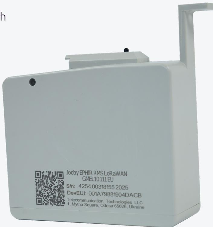
This radio module for Elster gas meters enables suppliers and management companies to receive accurate data on gas consumption as fast as possible. The device automatically collects meter readings and transmits the data to the server over a LoRaWAN wireless network at a preset interval. Once gathered, the data becomes
