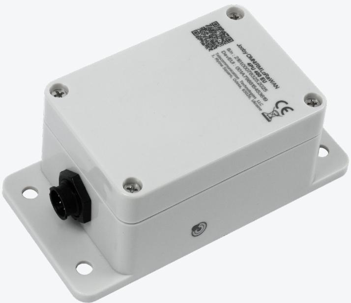
A pulse radio module enables utilities and management companies to receive up-to-date consumption data quickly. The device is connected to metering instruments via the appropriate sensor(s) and is activated automatically. Once activated, the radio module starts recording and transmitting counted pulses.
