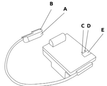
e) Sensor button for sending the current status of the radio module with sensor /
