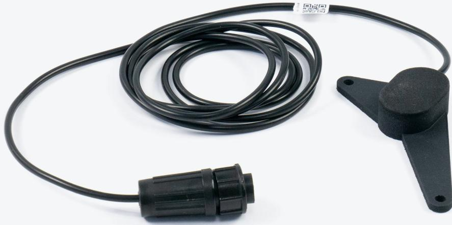
The inductive Sensor is designed to transmit data from analog water meters to the Jooby OMNI RM LoRaWAN 4PU 200 / 204 Pulse Radio Module. The device is mounted on the metering instrument housing and connected to the module. After installation, the Sensor begins to register the number of revolutions of the water meter's measuring pointer and transmits the data to the Pulse Radio Module.
