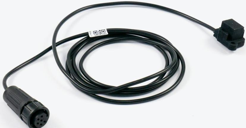
The magnetic Sensor is designed to transmit water-meter readings to the Jooby OMNI RM LoRaWAN 4PU 204 EU Pulse Radio Module. The Sensor is mounted on the meter housing and connected to the module. After installation, it records the number of revolutions of the water meter's built-in magnet, generates pulses with a specified coefficient, and transmits them to the Pulse Radio Module.
