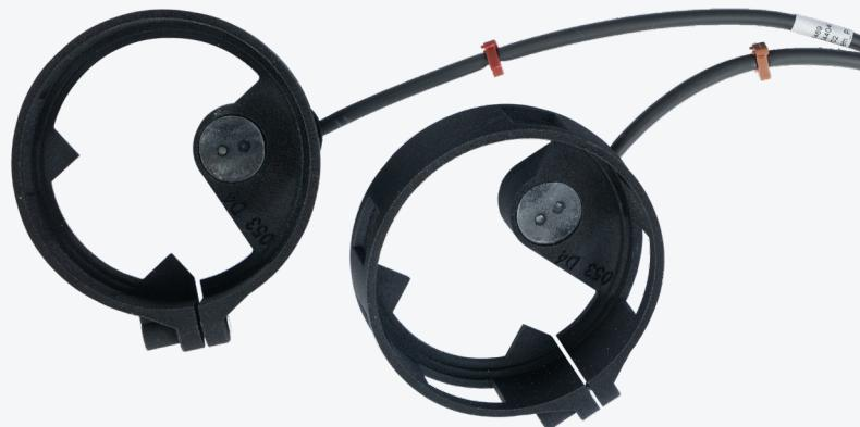
The optic sensor detects the rotations of the analog water meter's measuring pointer and transmits pulses (the number of pulses is a multiple of the number of revolutions by the pointer) to the Jooby OMNI RM LoRaWAN 4PU 204EU radio module.
