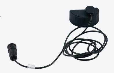
The optic sensor detects the rotations of the analog water meter's measuring pointer and transmits pulses (the number of pulses is a multiple of the number of revolutions by the pointer) to the Jooby OMNI RM LoRaWAN 4PU 204EU radio module.
