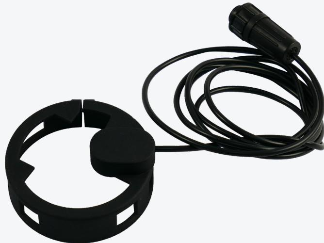
Optical sensor for transmitting data from analog water meters to the **Jooby OMNI RM LoRaWAN 4PU 200 / 204 / 205 EU** pulse radio module. The sensor is mounted on the meter case and connected to the radio module. The device starts counting the revolutions of the water meter's dial and transmits the data to the pulse radio module.
