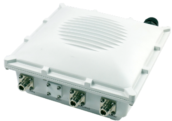
Figure 4: Hardware Interfaces – Bottom side of Jooby Gateway LoRaWAN 402 EU
