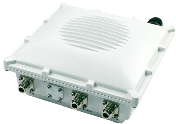
Figure 4: Hardware Interfaces – Bottom side of Jooby Gateway LoRaWAN 403 EU
