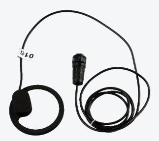
The inductive sensor is designed to transmit data from analog water meters to the Jooby OMNI RM LoRaWAN 4PU 200 / 204 / 205 EU Pulse Radio Module. The device is installed on the enclosure of the metering device and connected to the radio module. After that, the Sensor begins to record the number of revolutions of the water meter's measuring arrow and then transmits the data to the Pulse Radio Module.
