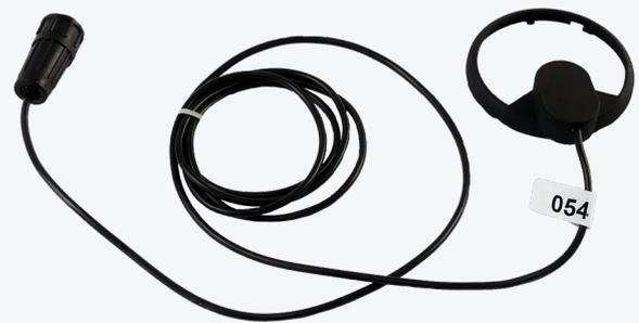
The inductive sensor is designed to transmit data from analog water meters to the Jooby OMNI RM LoRaWAN 4PU 200 / 204 / 205 EU Pulse Radio Module. The device is installed on the enclosure of the metering device and connected to the radio module. After that, the Sensor begins to record the number of revolutions of the water meter's measuring arrow and then transmits the data to the Pulse Radio Module.
