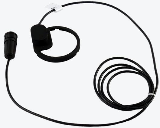
The inductive sensor is designed to transmit data from analog water meters to the Jooby OMNI RM LoRaWAN 4PU 200 / 204 / 205 EU Pulse Radio Module. The device is installed on the enclosure of the metering device and connected to the radio module. After that, the Sensor begins to record the number of revolutions of the water meter's measuring arrow and then transmits the data to the Pulse Radio Module.
