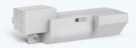
This radio module for Samgas gas meters allows suppliers and management companies to quickly get accurate data on the consumption of gas. The device automatically captures the meter readings and sends data to the server over a LoRaWAN wireless network at a defined frequency. The software then converts the data into readings and the information becomes
