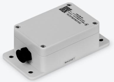
A radio module for various types of meters that enables supplier and management companies to get timely and relevant information about the resources their customers use. The device connects to meters using smart sensors and records metering pulses. The defined number of pulses is then transmitted to the server
