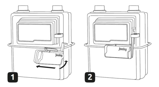
Make sure that the LED indicator on the radio module flashes once at the moment of installation. In addition, you should also see six short flashes within 1 minute. This means that a radio exchange took place between the radio module and the gateway.
